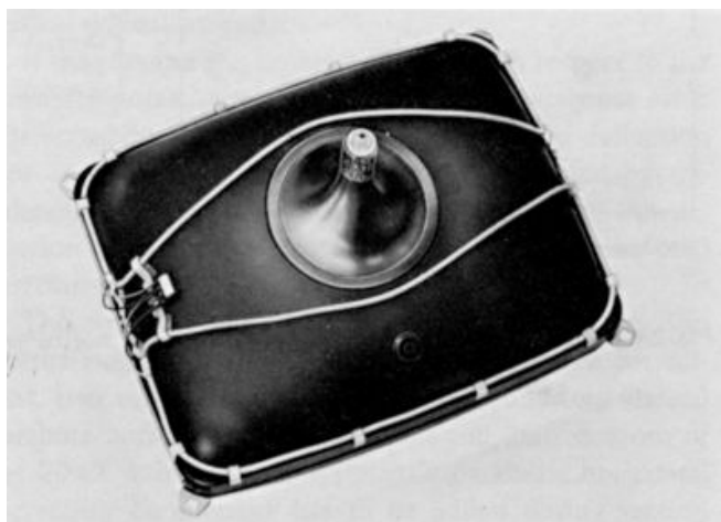
Fig. 22 — Positioning of degaussing coils on a 20AX tube.
